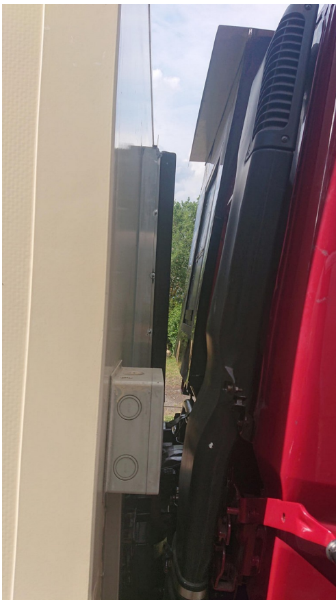
The driver's-cab can be easily tilted without having to release any locks and is still sealed
