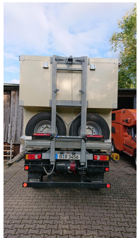
Motorcycle platform, electrically lowerable
