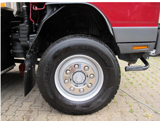
Stainless steel nut caps and protective ring
