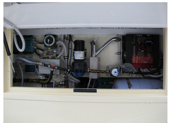
Service hatch right side outside with water and electrical equipment
