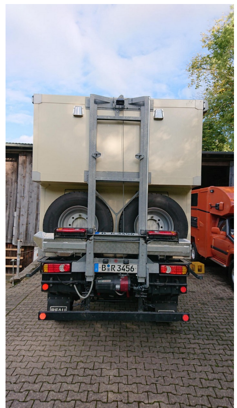
Motorcycle platform, electrically lowerable
